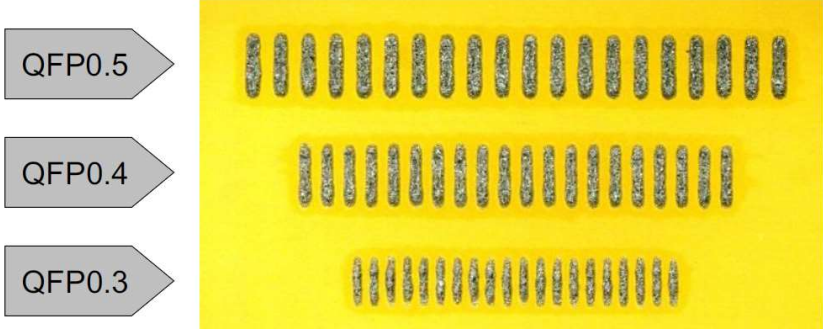
Print Results of QFP after the 5th Print Using a Nano-Coated Stencil (Area 1)
